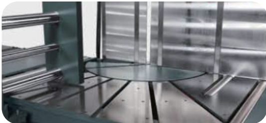
Heavy-duty miter-cutting work table & large scrape-free vise plates
