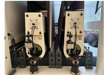
Eccentric structure to protect the sanding belt and roller
