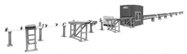
The GR series are machines designed for maximum output and processing quality in the minimum space possible. It can work with 6 or 12-meter-long bars and the material is moved by the means of a roller to optimize efficiency in a reduced space. Though the material is moved by a roller infeed, the customer can use GEKA's patented Minimal Waste System to ensure a minimum waste per bar, reducing the scrap to virtually zero.
