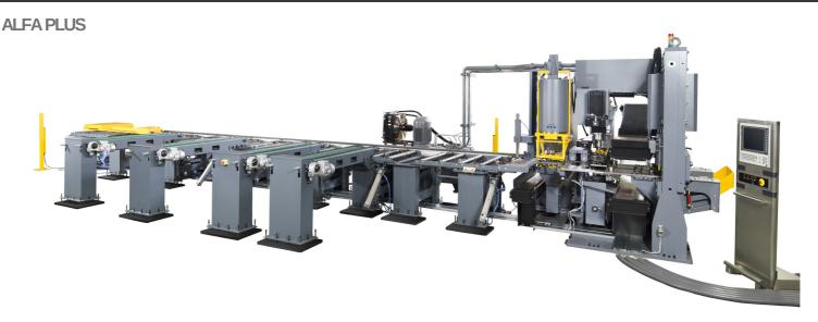
The ALFA PLUS not only includes the possibility of working with flat bars but also an angle bar. With this machine, a steel fabricator will be able to process both angles and flats to maximize their production output with all the same options as the smaller ALFA ranges. This machine will surpass the investment cost in no time with the additional options as the automatic infeed and outfeed.
