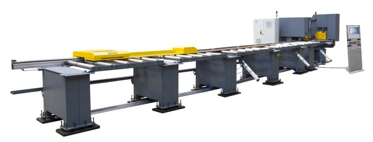
The ALFA series is a CNC punching and shearing machine specifically designed for steel fabricators that require medium and high output production. In the this ALFA version, the fabricatorwill be able to process flat bars from 6 to 12 meters and add a wde range of options like marking, drilling mitre shearing and automatic loading and unloading to increase take their production to a new level.
